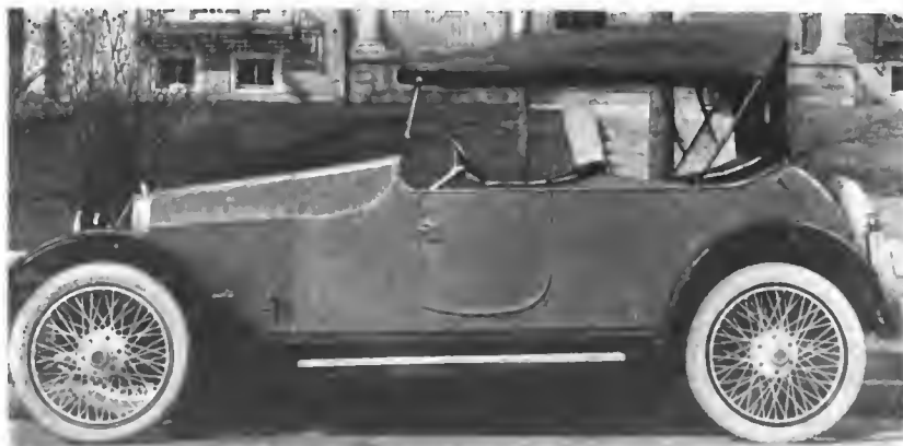
Side view of the four-passenger Scripps-Booth eight, showing semi-deck behind front seat. Note rounded rear carrying spare wheel
